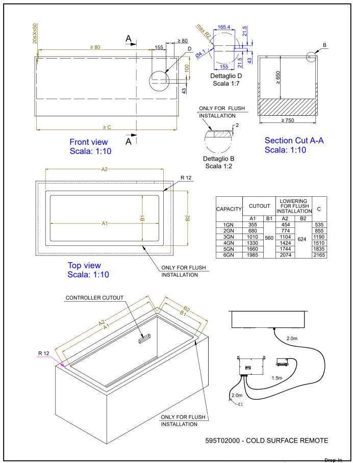
Drop-in remote refrigerated quartz surface (5 GN container capacity)
